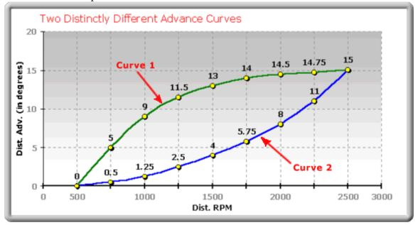
Therefore, the correct cam is the foundation for the correct advance curve. There are 18 different mainshaft cams used on the 23 Corvette TI distributors.
