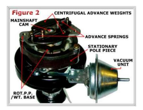
Since the distributor rotor is attached to the Rot.P.P./Wt. Base, and that assembly is moving clockwise relative to the mainshaft, the result is an advanced spark (Rot.P.P./Wt. Base rotation in degrees is equivalent to centrifugal distributor advance in degrees). In addition, the Rot.P.P./Wt. Base also determines the total amount of advance achievable. There are ten (10) Rot.P.P./Wt. Bases and three (3) styles of weights used on the 23 Corvette TI distributors.
